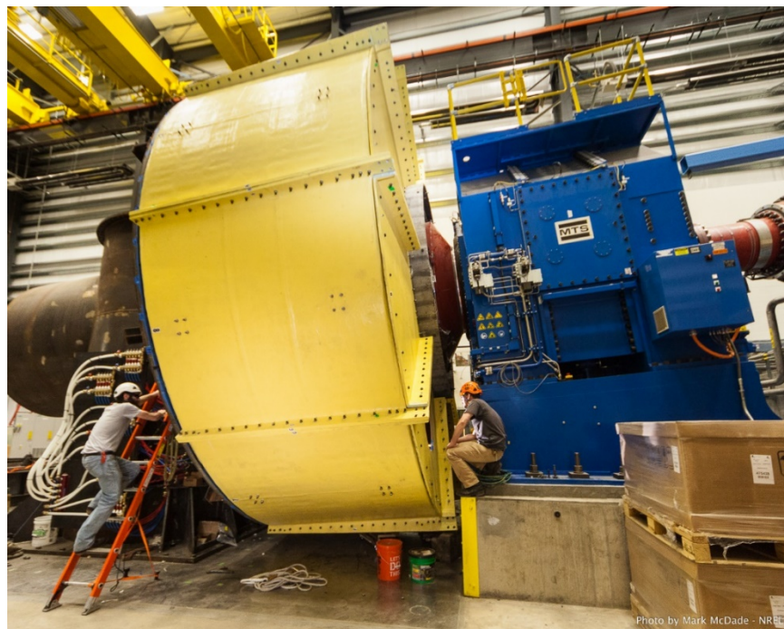
Columbia Power (C·Power) – Power Take Off Testing
