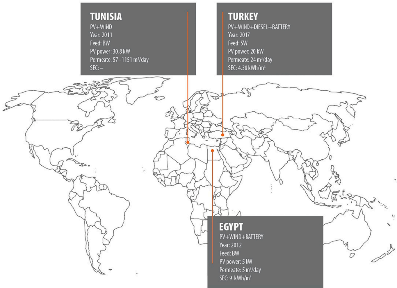
Fig. 9. Selected hybrid energy desalination installations worldwide (based on [171,179,255]).
