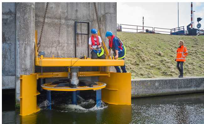
Fig. 2. 50kW turbine by Water2Energy demonstrated in the port of Flushing
