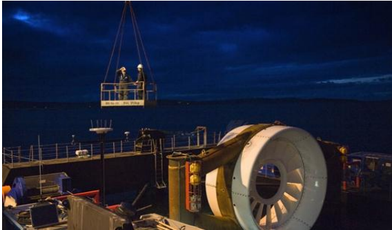
Figure 14b: Open Centre Turbine being prepared for deployment in Orkney (EMEC) [41]
