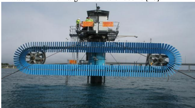
Figure 13a: Nereus Tidal Turbine [40]
