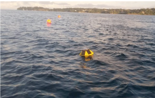
Fig. 2 Metoceanic buoy in the vicinity of Saboga Island. In the background, support, and signaling buoys can be observed. November 2022.
