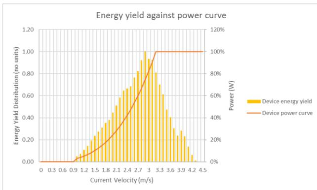
Fig. 6 Energy yield with the device power curve
