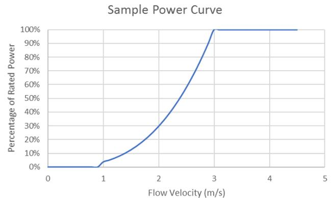
Fig. 1 – Example power curve for a tidal device
