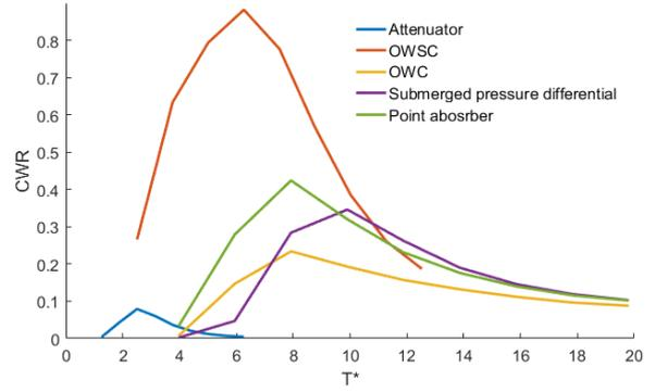
Fig 7: CWR against non-dimensional wave period.
