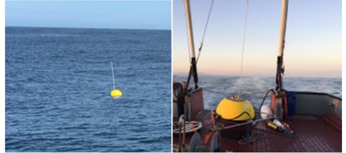
Fig. 2 Waverider buoys deployed in Lakeside, OR (#46260, left) and Fort Bragg, CA (#46263, right).
