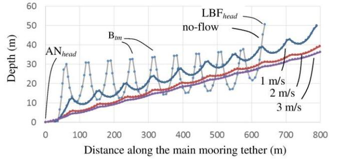
Fig. 9 Shapes of the example mooring tether of the design of Tab. IV when the 8-turbine array is under different flow speeds, as computed by a basic finite element model. Horizontal pulls were based on Tab. I. Vertical forces and fairlead depths correspond to data shown in Fig. 6.
