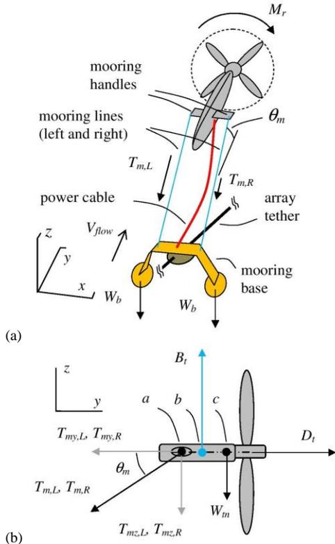
Fig. 2 (a) The single turbine mooring system with a turbine in its operational pose; (b) force analysis of the turbine in side view.
