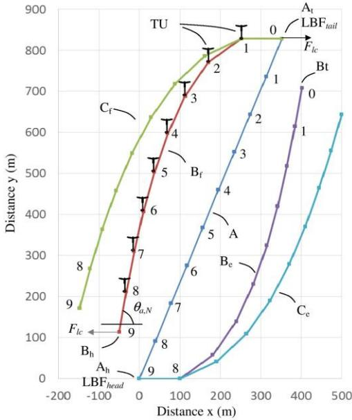
Fig. 8 Examples of 2D layout of a turbine array of the design of Tab. IV under different conditions.
