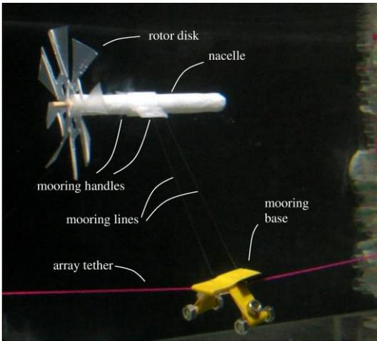
Fig.10 Close view of a model in the water tank under a flow of  $\sim 12$  cm/s ( $\sim 2$  m/s full scale).
