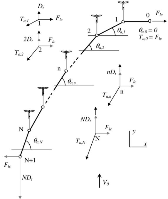
Fig. 7 Generalized 2D layout of a turbine array when deployed across stream, with force analysis.
