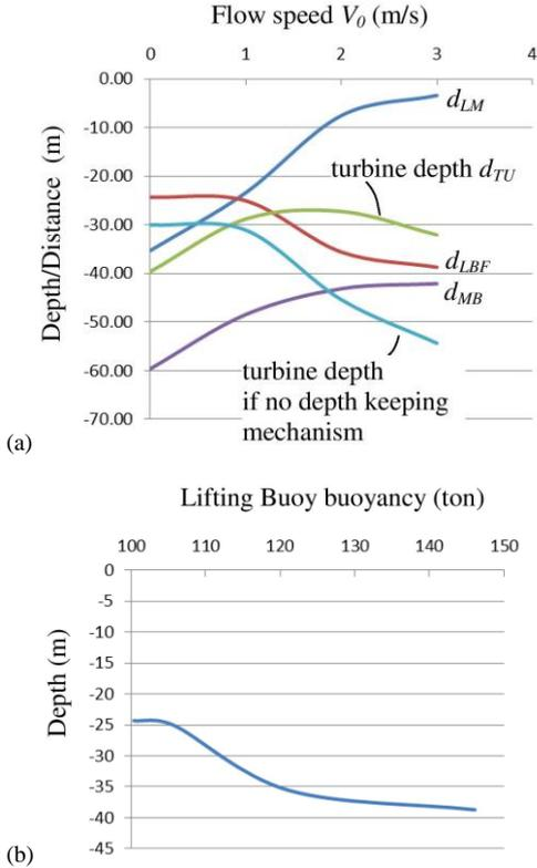
Fig. 6 (a) Estimated turbine depths in different flow speeds when the depth maintaining mechanism is applied, in comparison with the situation when no correction mechanism is used.  $d_{MB}$  is depth of the mooring bases on the array tether.  $d_{LM}$  and  $d_{LBF}$  see Fig. 4(a) and texts. (b) Buoyancy to depth relation of the corresponding lifting buoy design.
