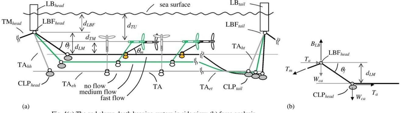
Fig. 4(a) The end clump depth keeping system in side view; (b) force analysis.
