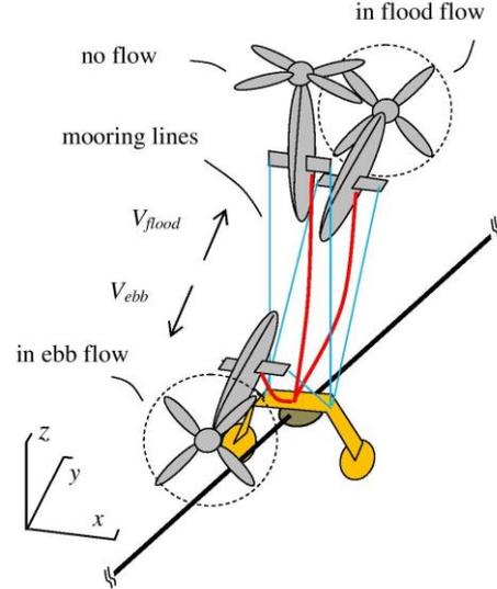
Fig. 3 Bi-directional operations of the single turbine mooring system
