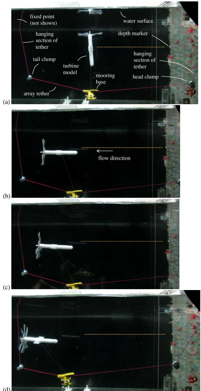
Fig. 11 Model tests of an end clump system for maintaining turbine depth; (a) no flow, (b) flow speed  $\sim 6$  cm/s ( $\sim 1$  m/s), (c)  $\sim 12$  cm/s ( $\sim 2$  m/s), (d)  $\sim 18$  cm/s ( $\sim 3$  m/s).
