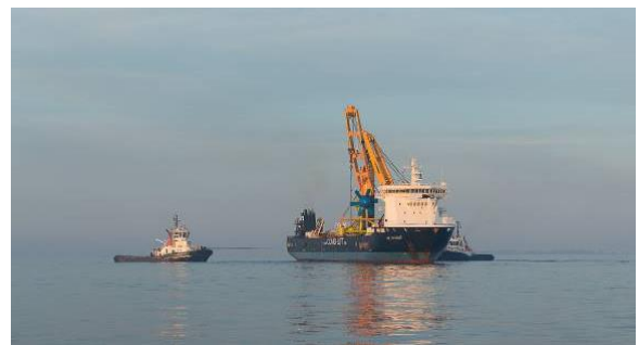
Fig. 8 Heavy Lift Vessel used for the initial installation
