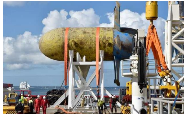
Fig. 11 D10 's turbine on ifs offshore berth after retrieval
