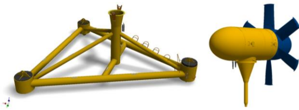
Fig. 2 Interface between the GBS and the turbine
