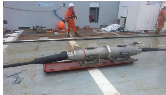
Fig. 4 D10's initial dry mate connector on its guiding plate
