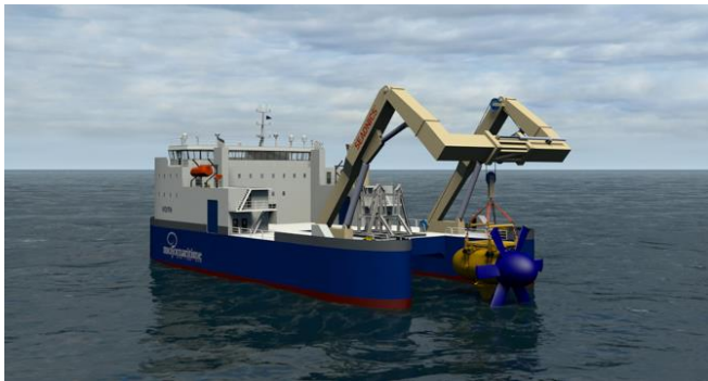
Fig. 15 MOJO MARITIME HF4 vessel lifting Sabella D10 turbine
