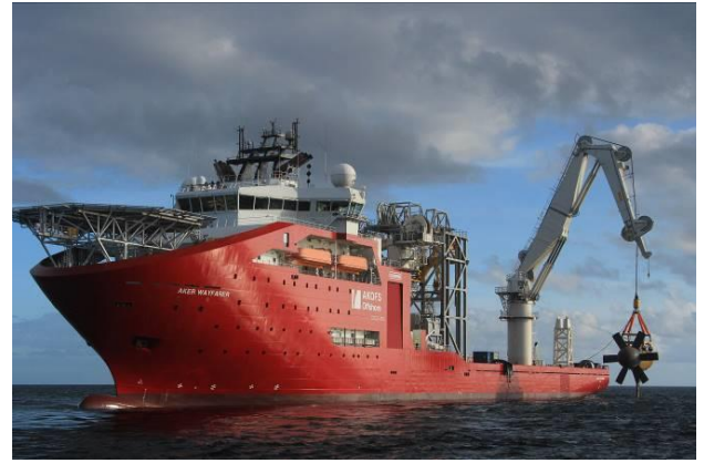
Fig. 10 Sabella D10 's turbine retrieval in July 2016
