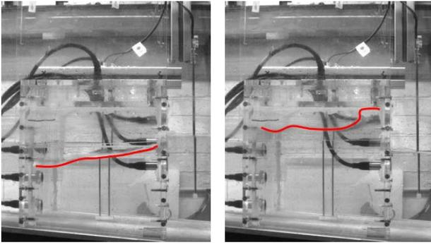
Figure 8 Medium sloshing water column behaviour with solid red line showing the water surface
