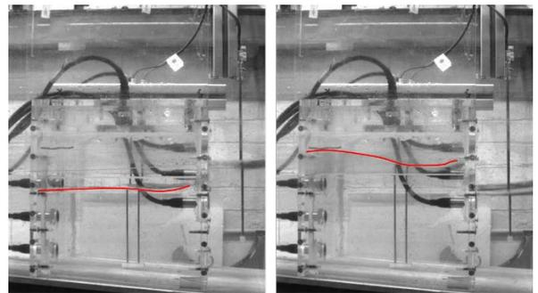
Figure 7 Low sloshing water column behaviour with solid red line showing the water surface
