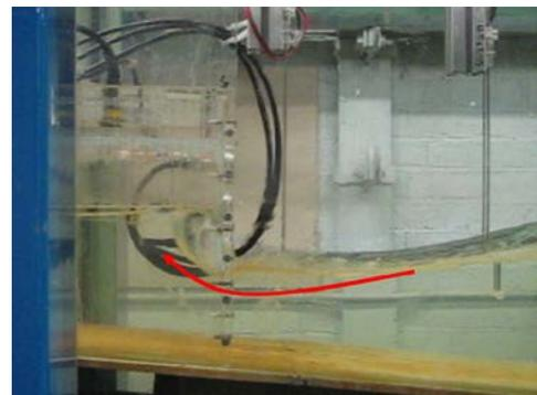
Figure 12 Venting phenomenon where the water level fell below the chamber opening and air enters the chamber through the front opening indicated by the solid red arrow.
