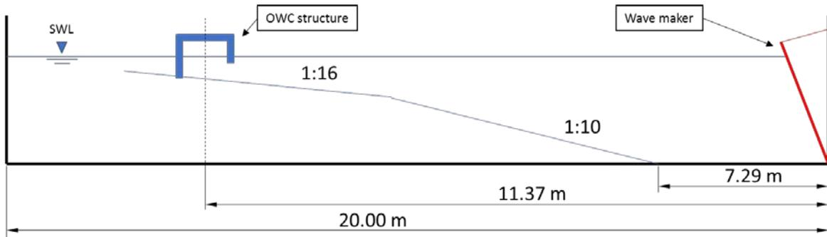
Figure 1 Schematics of the long wave flume and the model structure location with dimension shown in metre.
