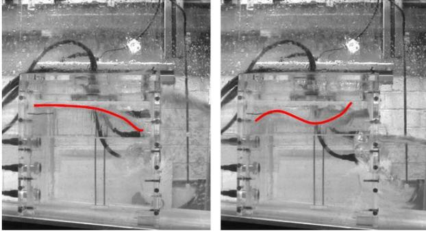
Figure 9 High sloshing water column behaviour with solid red line showing the water surface
