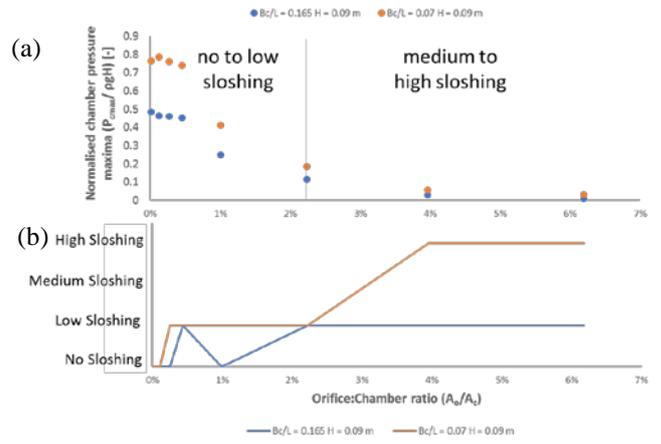
Figure 10 (a) Chamber pressure maxima measurement for  $B_c/L = 0.165$   $H = 0.09$  m (blue circle) and  $B_c/L = 0.07$   $H = 0.09$  m (orange circle) vs orifice:chamber area ratio; (b) sloshing status for the same colour data points vs orifice:chamber area ratio
