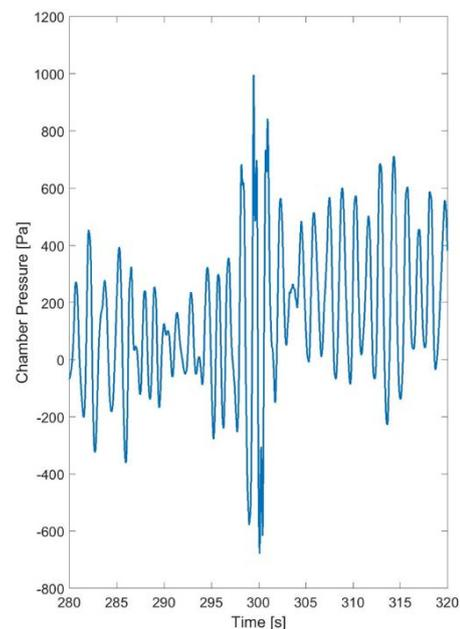
Figure 13 Time history chamber pressure measurement during the venting event.
