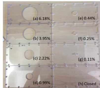
Figure 4 Various orifice openings used for the experiment with orifice:chamber area ratio of (a) 6.18%, (b) 3.95%, (c) 2.22%, (d) 0.99%, (e) 0.44%, (f) 0.25%, (g) 0.11%, and (h) Closed (0.0%).
