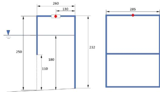
Figure 3 The cross-sectional image of the physical model used with detailed dimension of the chamber in mm. Solid red diamond shows the position of the pressure transducer used.
