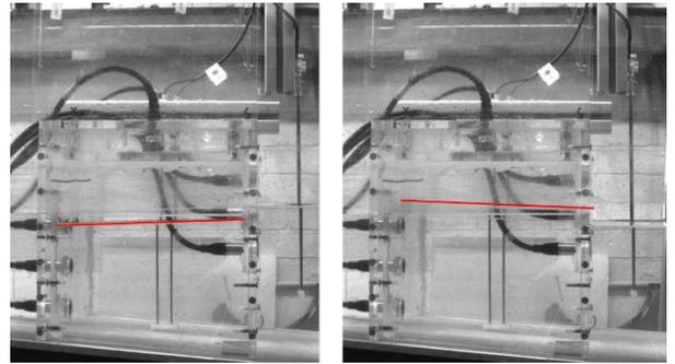
Figure 6 Well behaved (no sloshing) water column behaviour with solid red line showing the water surface
