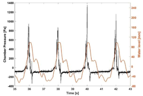
Figure 11 Time history chamber pressure measurement on the chamber ceiling (left y-axis, black) and chamber water column elevation (right y-axis, orange) at the same time step.
