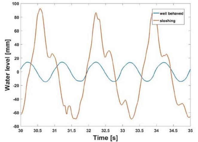
Figure 5 In-chamber water column movement for the well behaved (blue) and sloshing (orange) conditions in mm.
