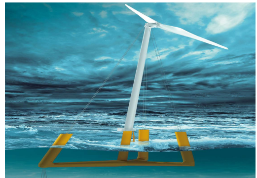
Fig. 9. Schematic of the 3.0 MW SCD@-Nezzy floating wind turbine [30]
