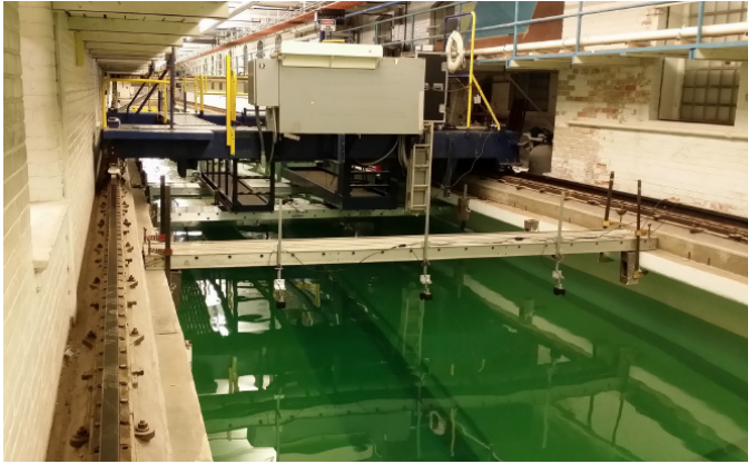
Fig. 4. Marine Hydrodynamics Laboratory tow tank and carriage [12].
