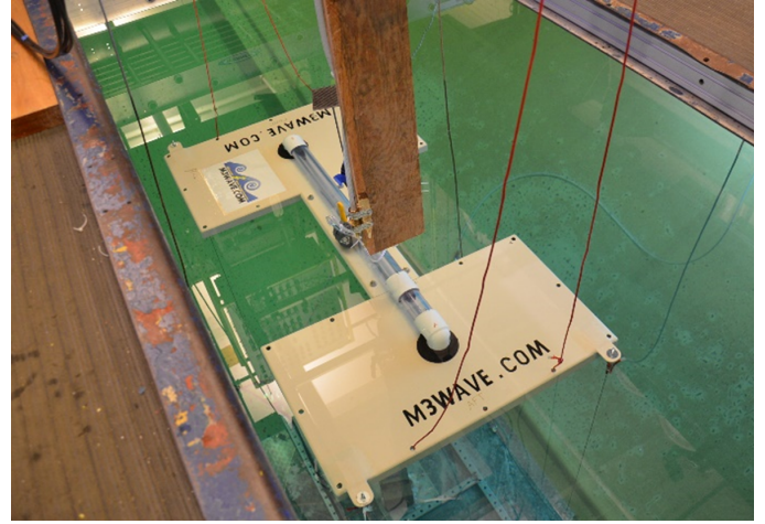
Fig. 5. Scaled M3 device installed in the tow tank [12].
