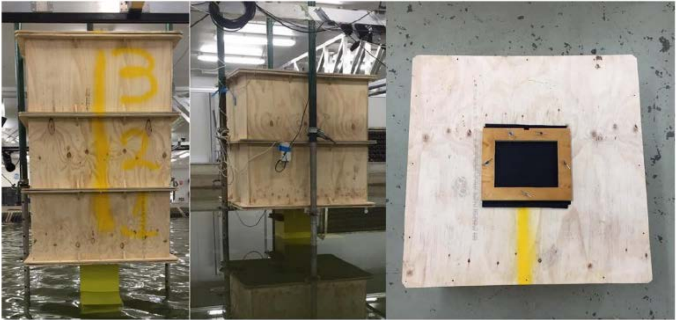
Fig. 3 Model scale OWC device fitted with additional 1.5 m 3 air chamber (left), 1 m 3 air chamber (middle) and PTO simulant secured using sealing plate (right)
