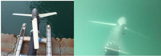
Figure 1. Scaled tidal turbine under field test.
