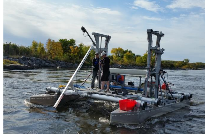
Figure 1 - ADCP measurements performed at the CHTTC site upstream of the 22-kW Mavi turbine measure the inflow. The ADCP is connected to the front of the turbine using a custom mounting bracket attached directly to the unit
