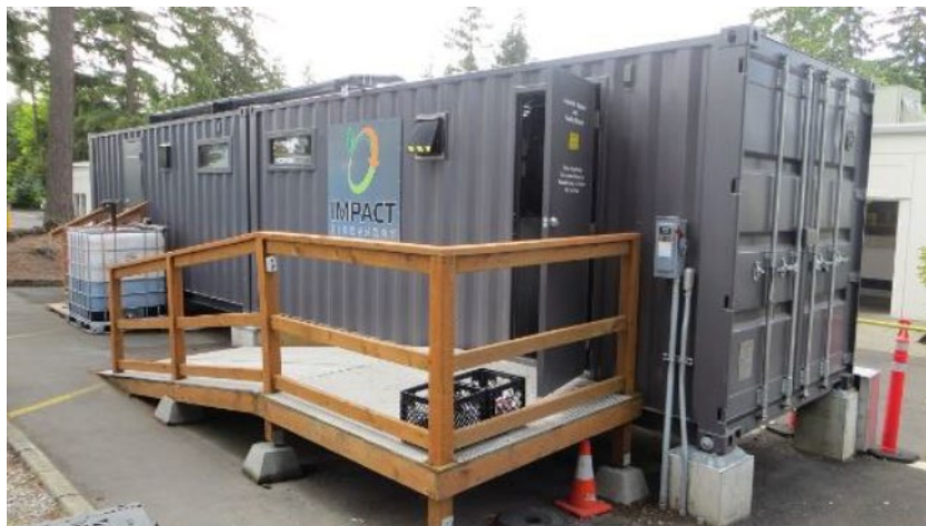
Figure 3.2. Impact Bioenergy modular anaerobic digestion system.
