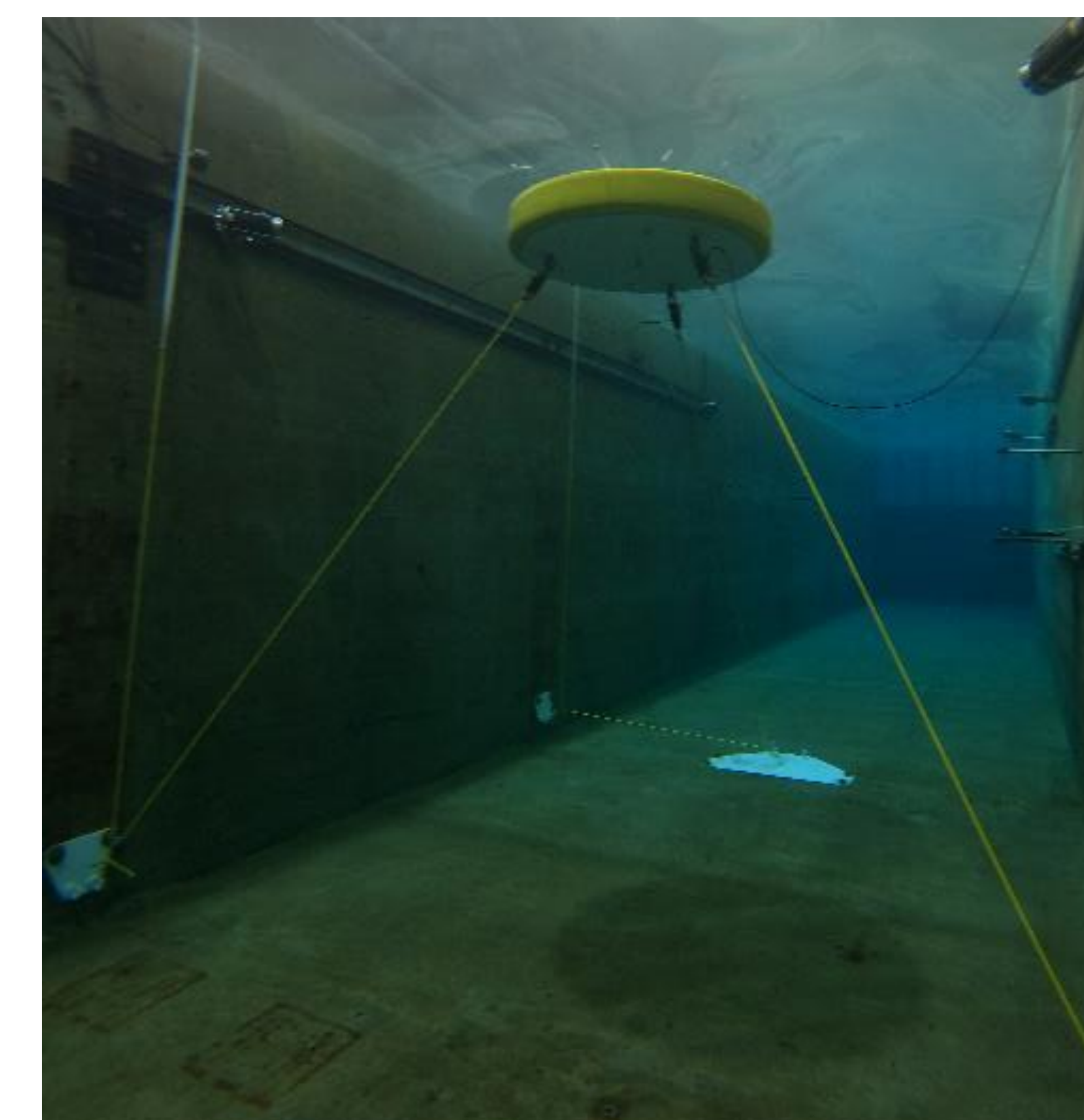
Figure 4: SubWEC three tether experimental set-up.
