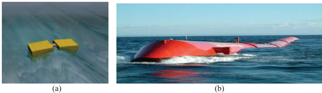
FIGURE 10. (a) Concept of Attenuator (b) Pelamis (Sea Snake) Wave Converter [21]
