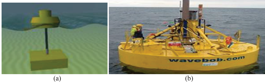
FIGURE 11. (a) Concept of Point Absorber (b) The Point Absorber[21]
