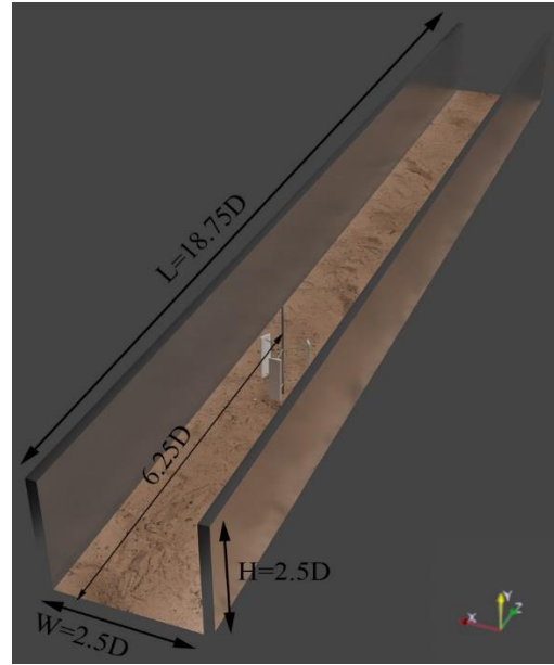
Figure 1: Schematic of the VAT, located 6.25D downstream of the inlet. Dimensions are normalized with the rotor diameter D(=2m) .
