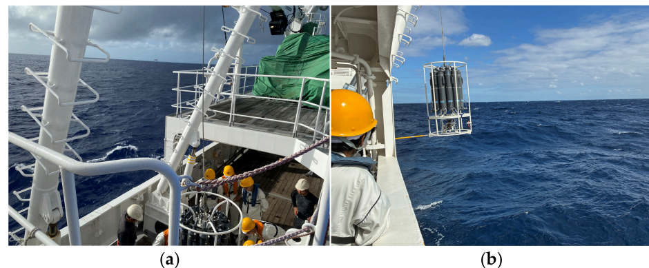
Figure 2. (a) Preparation of observation work. (b) CTD released into the sea.
