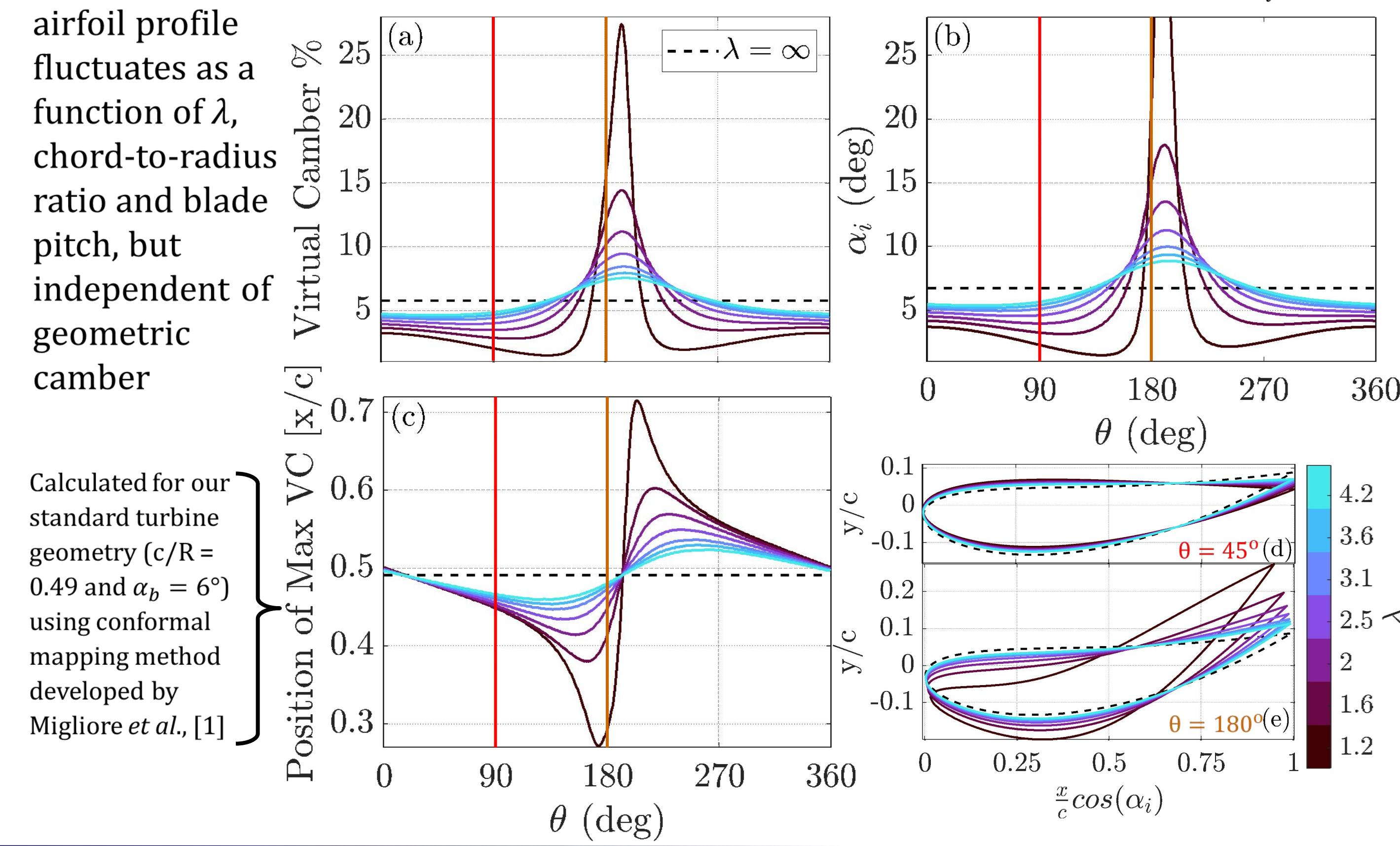
Calculated for our standard turbine geometry ( $c/R = 0.49$  and  $\alpha_b = 6^\circ$ ) using conformal mapping method developed by Migliore et al., [1]
