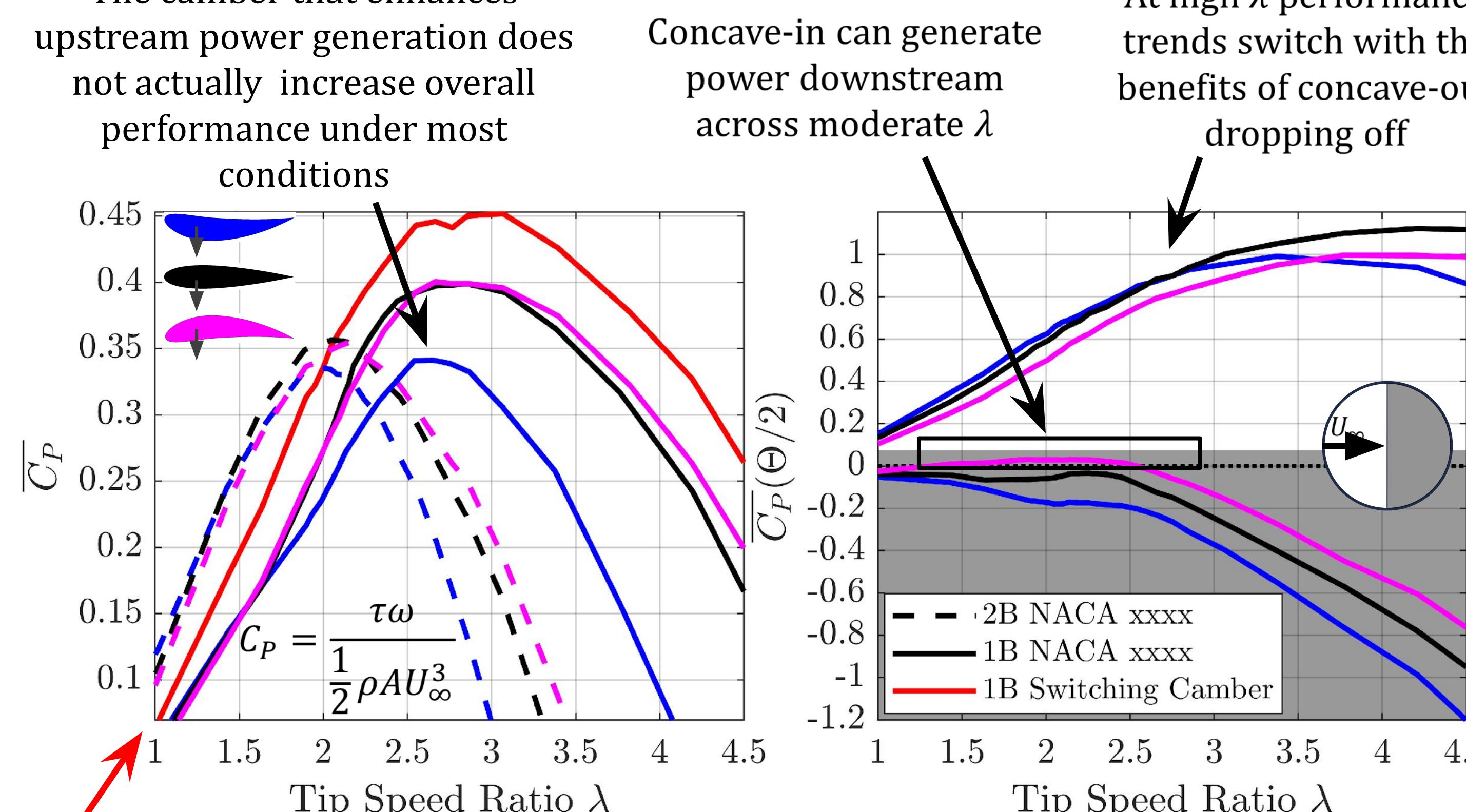
Red line, actively cambering through the cycle (averaging the best profile upstream and downstream) one blade turbine can improve efficiency relative to the symmetrical blade by 10-45%
