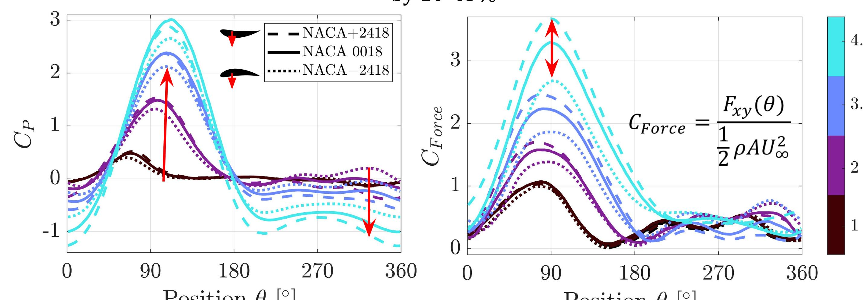
Concave-out performs better at the peak for below-optimal  $\lambda$  but has increased losses through the cycle. Concave-in is consistently worse upstream but is compensated by downstream improvement
