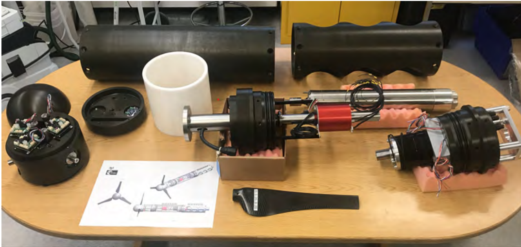
Figure 7: An image of the AFT components prior to assembly. The components are laid out with those located forward on the system being on the left side of the image. The housings are located near the top of the images.
