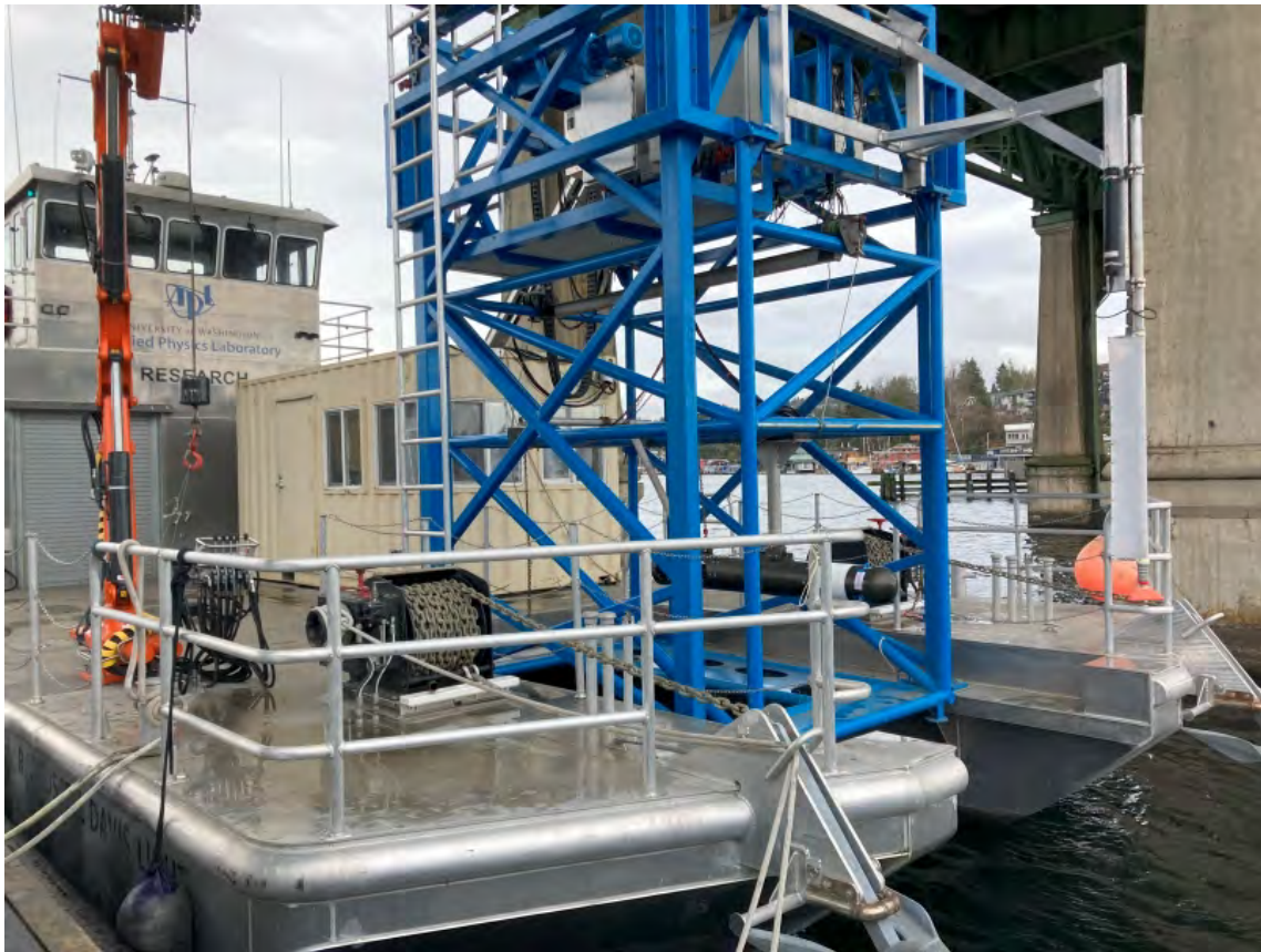
Figure 1: R/V Russell Davis Light with the AFT installed (without blades). The plume frame on which the AFT is mounted is lowered into the water during testing.
