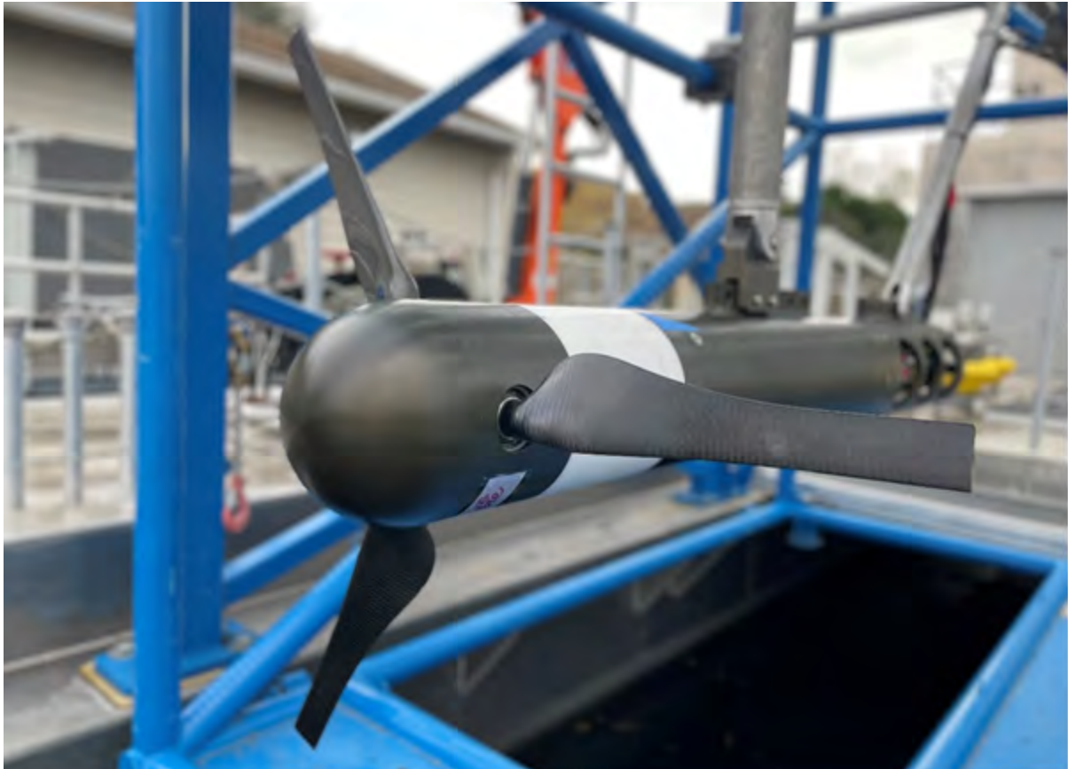
Figure 12: Photo of the field-scale AFT installed on RDL in preparation for system commissioning.
