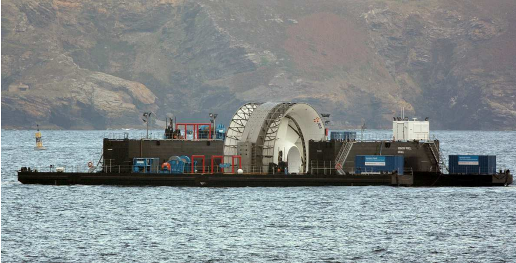
Figure 5 : Tidal turbine deployment barge
