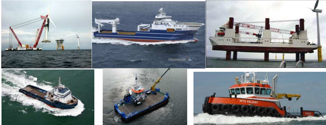
Figure 2 : Example offshore vessels (clockwise from top left) Rambiz HLV 1 , North Sea Giant OCV 2 , Resolution jackup barge 3 , MTS Valiant workboat 4 , Eurocarrier 2209 multicat 5 and Sea Cheyenne AHT 6
