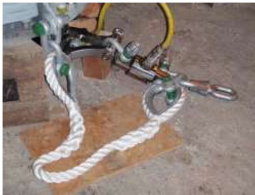
Figure 5: Example safety rope used on one mooring connection point of the SWMTF
