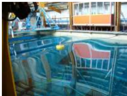
Figure 7: (left) 1:5 scale model of the SWMTF tested in the salt water basin at IFREMER (right) quasi-static analysis of the scale model mooring system conducted as part of the MERiFIC WP3.5 [28,29]. Measured and simulated values are shown as asterisk and square markers respectively
