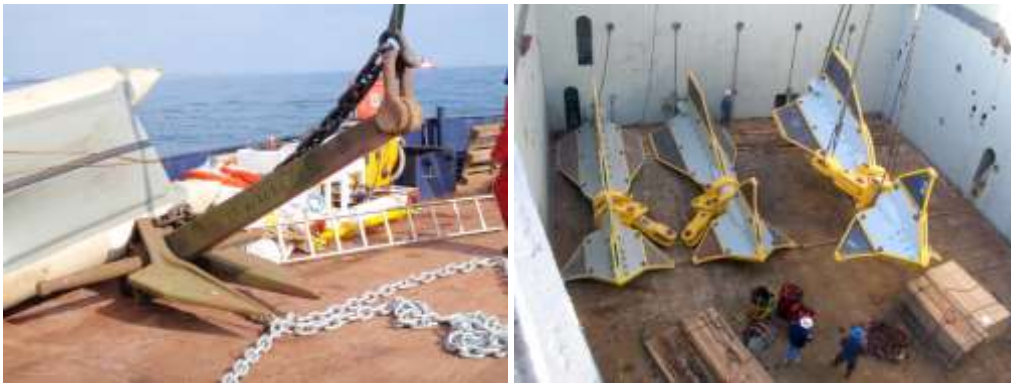
Figure 4: (left) 1.1 Tonne Danforth fluke anchor prior to deployment with the South West Mooring Test Facility 4 , (right) vertically loaded Delmar OMNI-Max anchor (source: Delmar Systems Inc.)
