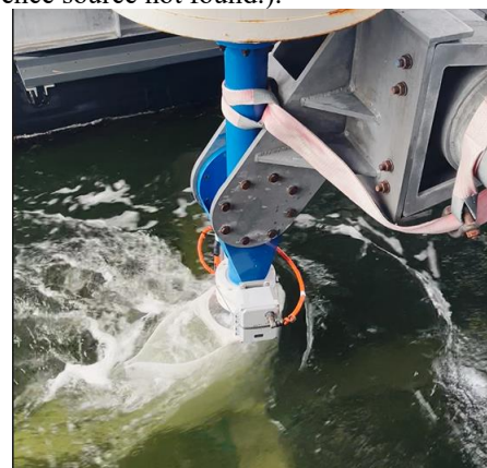
FIGURE 13: INSTRUMENTATION MAST AND FAIRING DEPLOYED WITH TURBINE BRAKED (I.E., NOT ROTATING). PHOTO BY MICHAEL MONAHAN / UNH.
