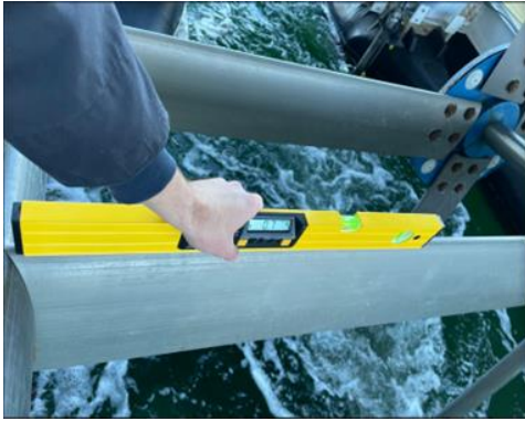
FIGURE 14: ELECTRONIC LEVEL ON THE BLADE STRUT (HORIZONTAL) USED TO ALIGN THE INSTRUMENTED BLADE (VERTICAL). PHOTO BY MICHAEL MONAHAN / UNH.
