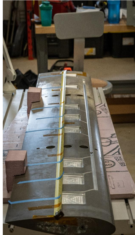
FIGURE 7: WIDE VIEW OF OUTER SIDE OF NEW ENERGY BLADE AFTER MACHINING SHOWING STRAIN GAUGE RECESSIONS AND WIRE ROUTING CHANNEL. PHOTO BY ANDREW SIMMS / NREL.
