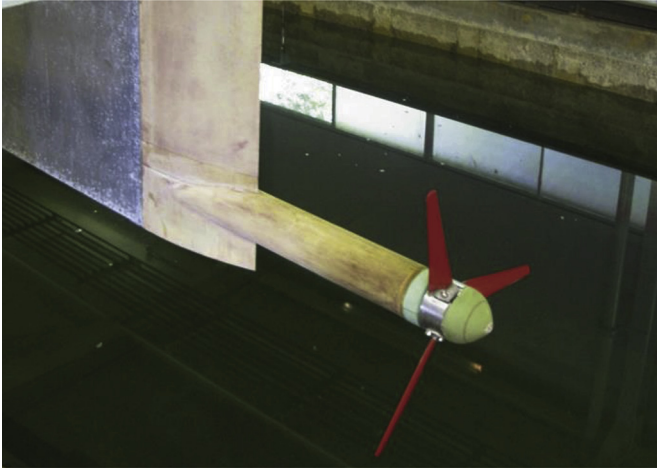
Fig. 4. Model tidal turbine prior to installation on the auxiliary carriage.
