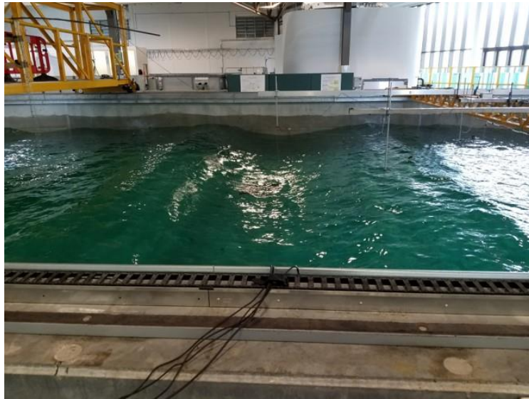
Figure 4: CalWave Device installed in the basin including the tanks wave sensor setup. Here, the device response and loads on the device during a severe sea irregular wave case was assessed. Equivalent wave heights of up to 22m occurred during the full length of the test.
