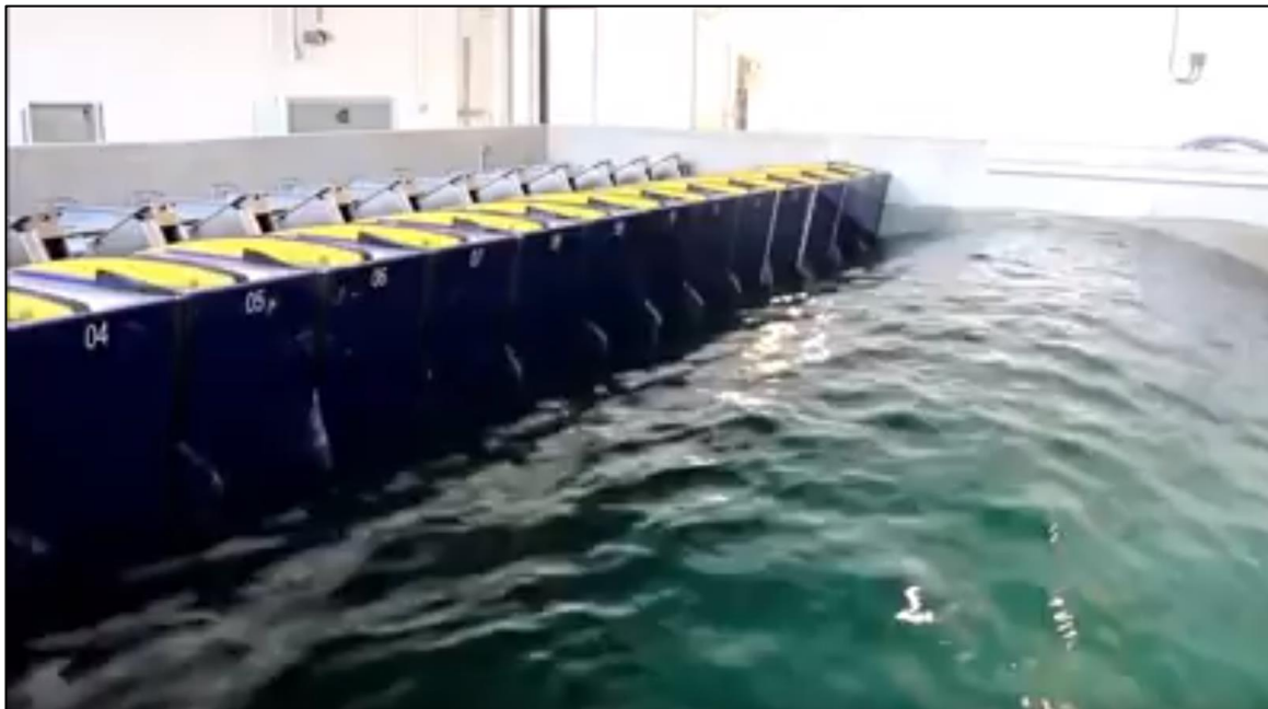
Figure 2: Wave Maker at the LIR Deep Ocean Basin
