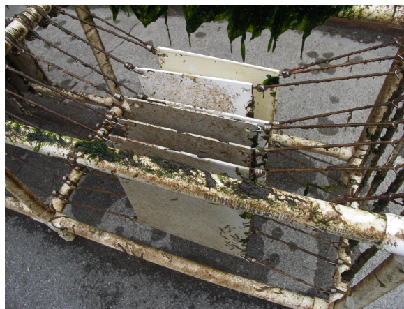
Figure 2. 8 x 8 in. coupons mounted within a PVC frame.
