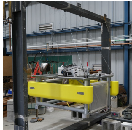
Figure 2. Swing test of the FOSWEC at HWRL to characterize mass and moments of inertia
