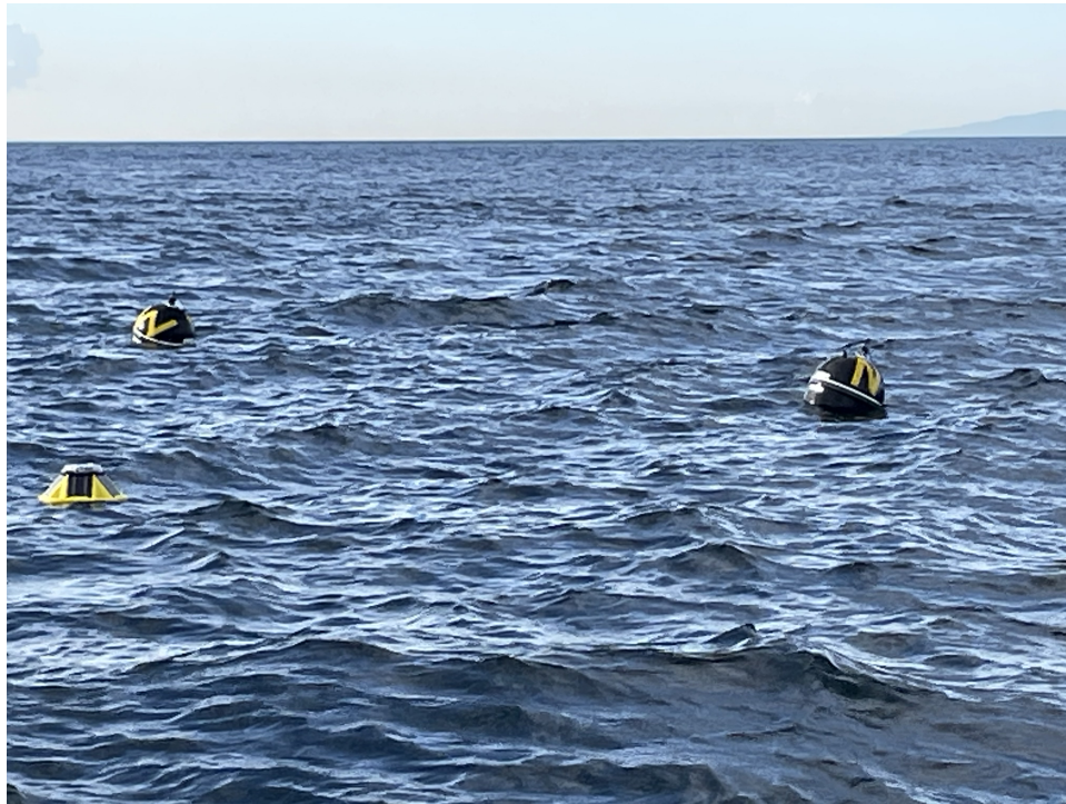
Figure 5. The WEC-buoy (left top), no WEC-buoy (right), and Sofar Ocean Spotter 3 buoy (left bottom) during a field test.
