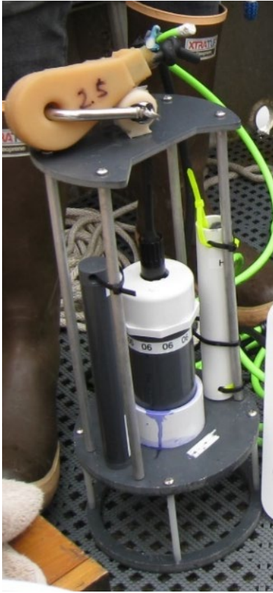
(a) Baseline C-DAISY and W-DAISY hydrophone holster (without fairing)
