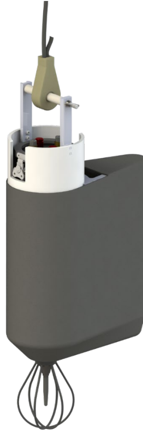
(b) Proposed C-DAISY hydrophone assembly with fairing and hydrophone guard
