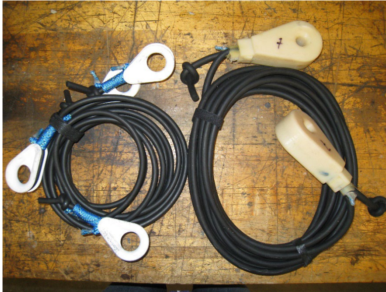
Figure 27: Rubber cords and termination – (left) prior to potting (right) after potting terminations in urethane
