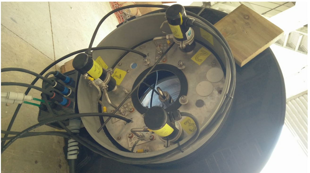
Figure 3 - Waveram 'Wavestaff' internal free surface monitoring gauges
