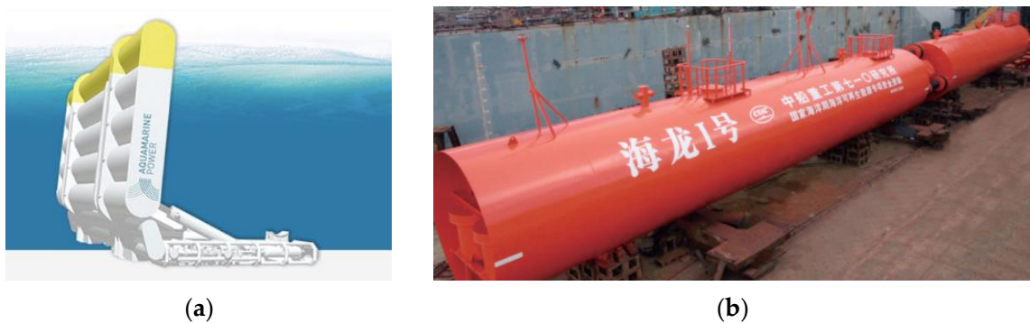
Figure 9. Applications of pendulum type and raft type WECs: the (a) Scottish pendulum "Oyster" [5] and (b) "Hailong #1" raft type WEC.
