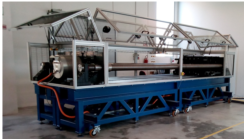
Figure 4. EMU installed on the HIL test rig at VGA facilities.
