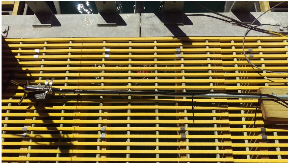
Figure 4.6: Temporary mount used for the first field deployment of an ADV on the turbine deployment platform on 6/15/18
