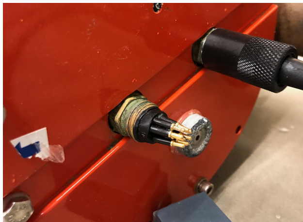
Figure 5.5: Damage to the ADCP bulkhead that was installed at the stern of the turbine deployment platform
