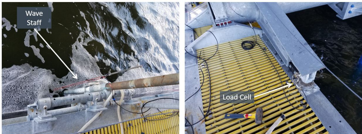
Figure 4.3: Wave staff (left) and load cell (right) during the mobile DAQ field test on the turbine deployment platform
