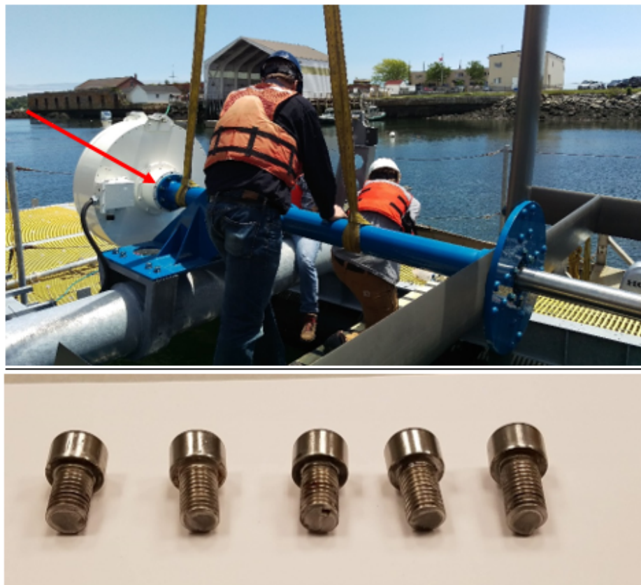
Figure 5.2: Stainless steel bolts sheared in the generator during turbine operation, the location of the bolts is indicated by the arrow in the picture of the turbine
