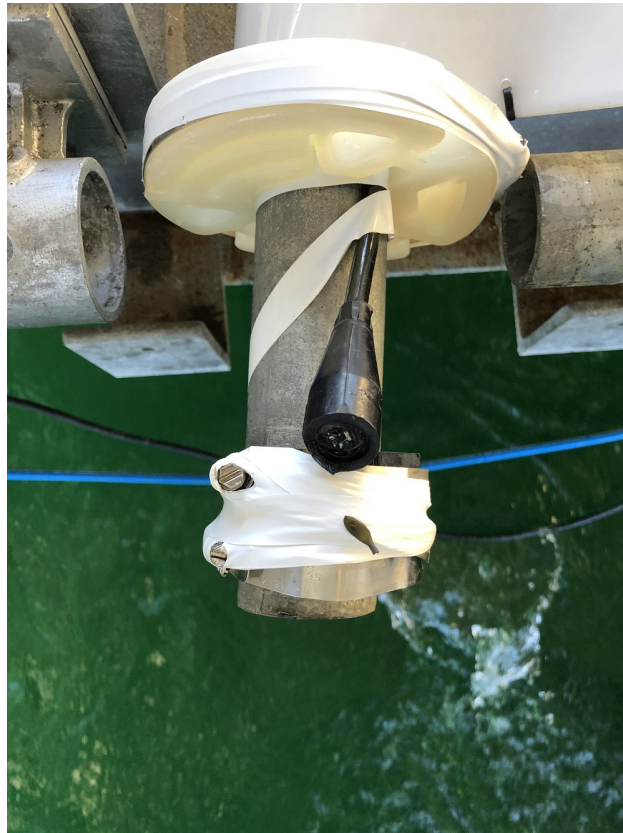
Figure 5.6: Damage to the ADV probe head on 2/4/19
