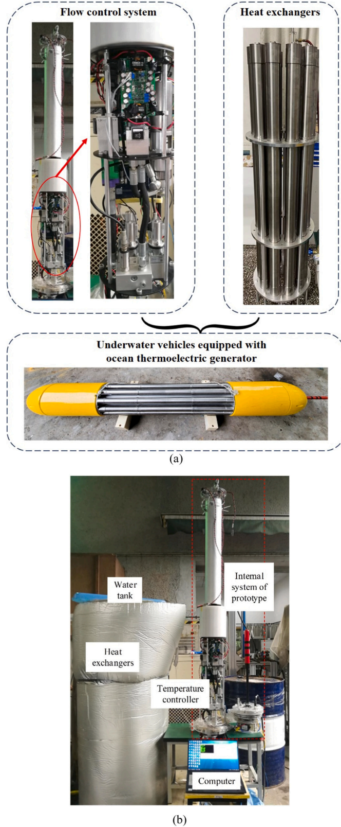
Fig. 8. Physical image of the (a) prototype and (b) the corresponding experimental set-up.
