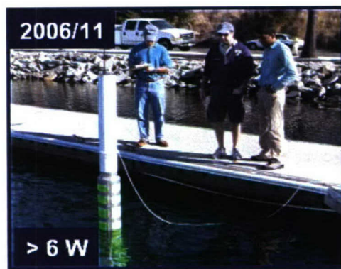
Fig. 18. 2.3-second spar and linear generator device in the water
