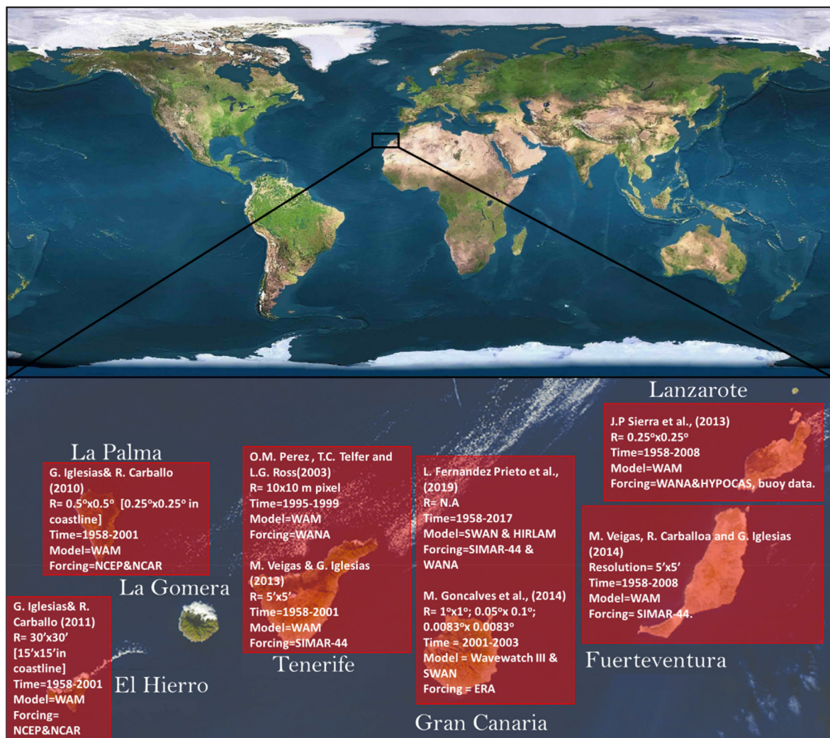
Fig. 1. Summary of the analysis of the wave resource in the Canary archipelago researches.
