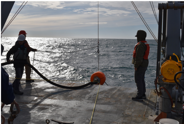
(c) The buoy trails behind as ship steams ahead, EM cable and stretch hoses are fed aft, and buoyancy elements are transferred over the transom with the A-frame and released.
