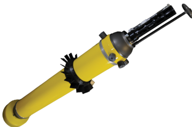
Figure 23. Photo of the Teledyne Marine APEX Current Profiling Float which utilizes a vane ring to generate rotational motion during a profile, which is involved in a process of directly measuring water current using motionally-induced electric fields.
