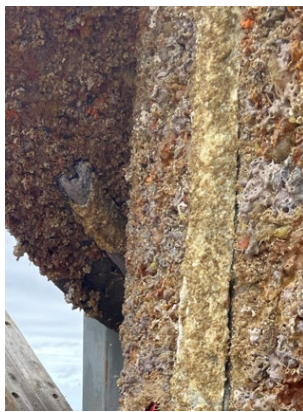
Figure 14 – Cathodic protection on the foundation after 2.5 years of immersion (Non coated areas)
