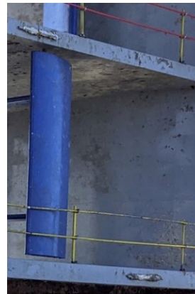
Figure 15– Cathodic protection on the turbine after 2.5 years of immersion (Coated areas)
