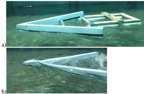
**Figure 8 :** Barrier 2A in: a) 2 m/s flow; and b) 3 m/s flow.
