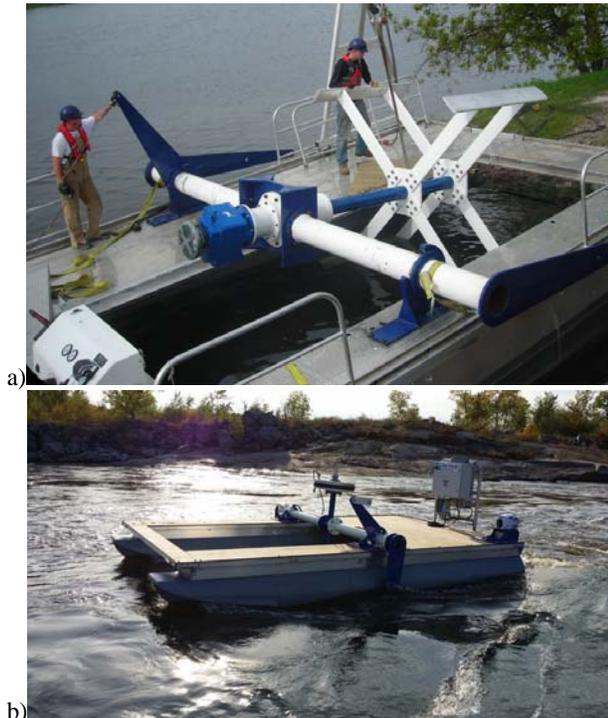
**Figure 2 :** New Energy vertical axis turbine: a) before deployment; b) operating in a fast-flowing river.
