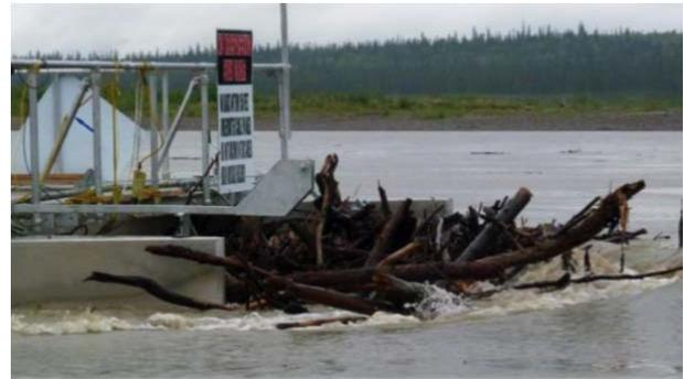
**Figure 1 :** Pile up of surface debris at a floating EnCurrent hydrokinetic turbine deployed at Eagle, Alaska (source: [2])
