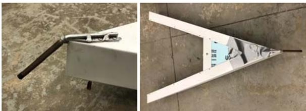
**Figure 9 :** Model Barrier 2B with rotating deflector bar.
