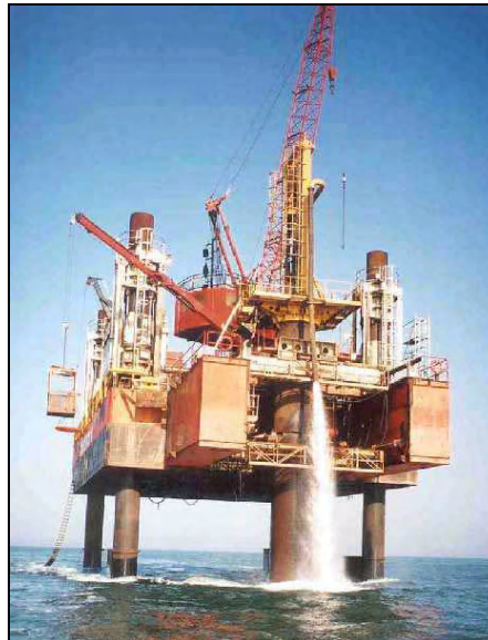
Figure 2.6 An example of a jack-up barge; Seacore Ltd's 'Deep Diver', photographed during the installation of MCT's 'Seaflow' turbine off Lynmouth in the Bristol Channel [2.6].
