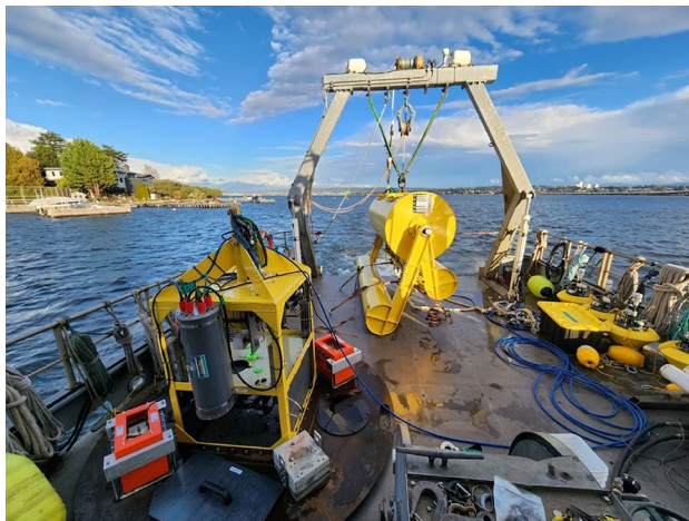
Fig. 3. Layout of TigerRAY components during transit on the back deck of R/V Jack Robertson. Picture taken by Curtis Rusch from February 2023 drifting tests.
