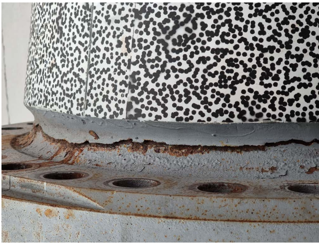
Fig. 6. Image of failed blade root showing crack from delamination extending around the circumference of root connection.
