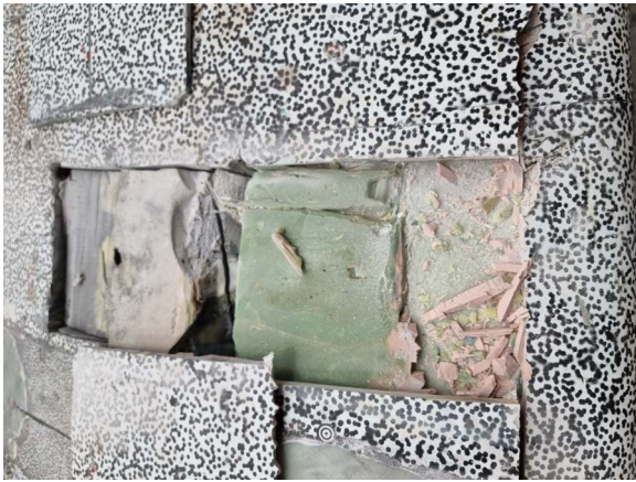
Fig. 14. Image showing a section of blade with the outer skin removed. From bottom to top: leading edge of blade, pink coloured filler at overlap seam, green Spabond adhesive, black carbon spar.
