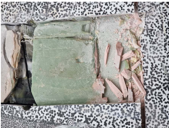
Fig. 15. Section through blade skin showing voids in between adhesive bond lines. Adhesive thickness at this location is approximately 15 mm.
