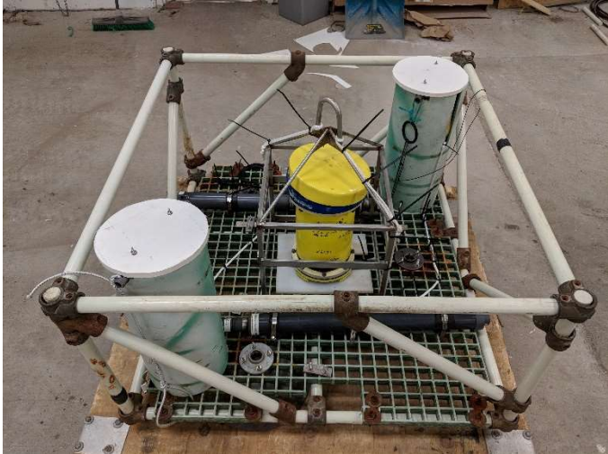
Figure 15 - ADCP frame deployed near the experiment, equipped with two acoustic releases and floats.
