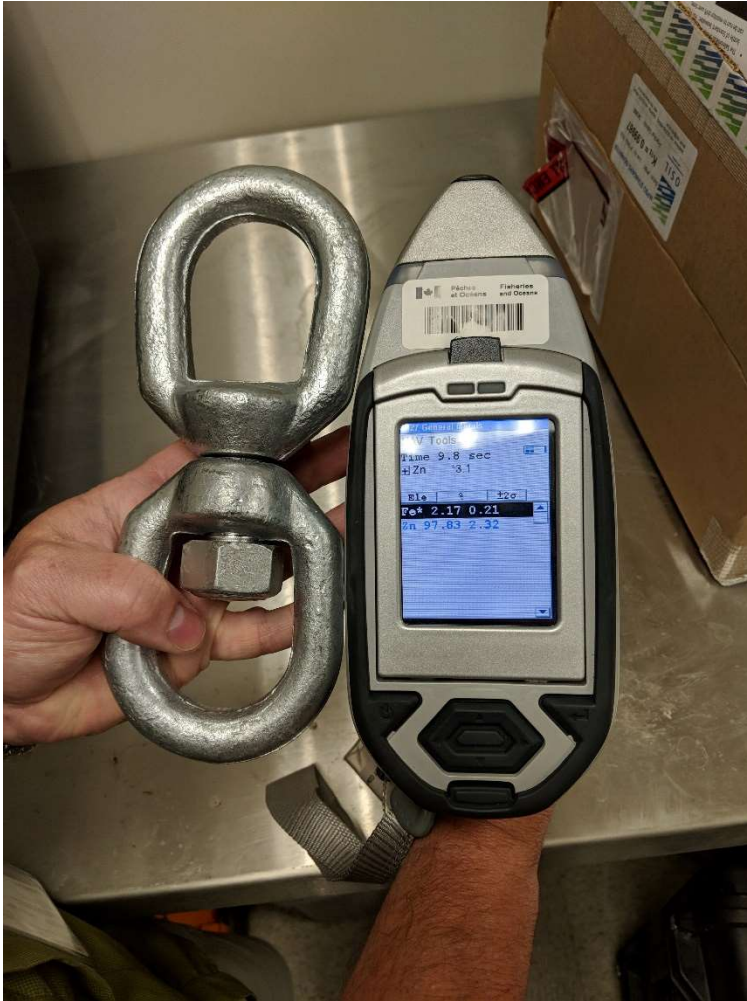
Figure 24 - XRF spectrometer showing elemental makeup of swivel.
