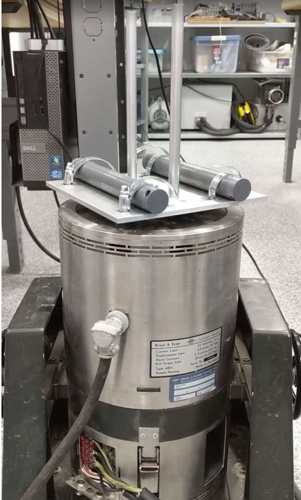
Figure 13 - Lowell MAT-1 data loggers mounted to shaker table.
