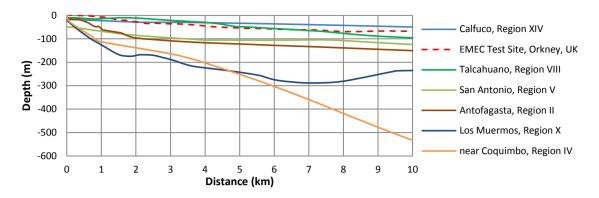
Figure 24: Comparison of seabed profile for Orkney, UK and Region IV of Chile
