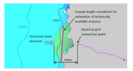
Figure 46: Methodology for approximation of technical wave resource
