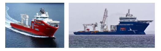
Figure 34: Dynamic Positioning (DP) vessels deployed at EMEC's tidal test site to install tidal turbines and support structures
