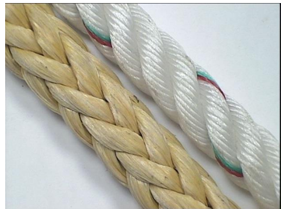
Figure 2. Examples of twisted and braided rope constructions
