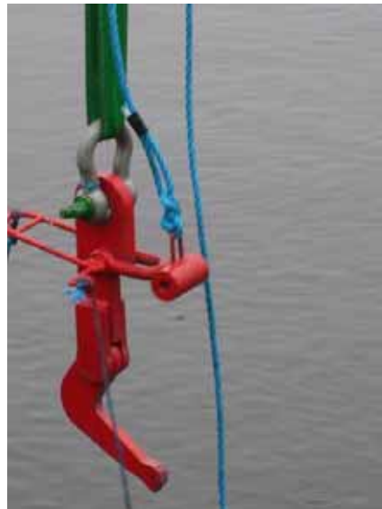
Figure 7.2: Mechanical release system.
