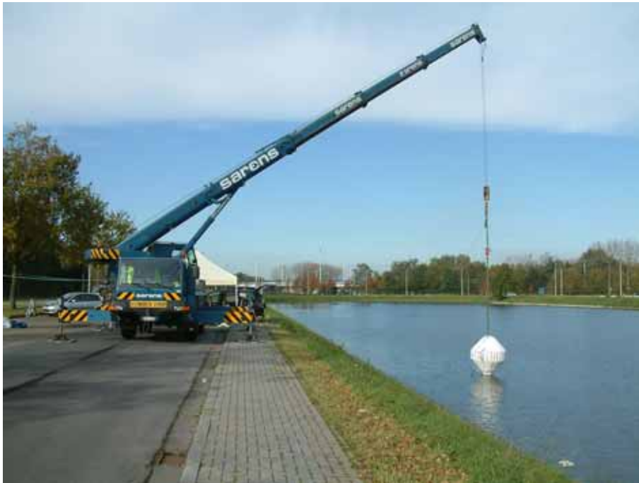
Figure 7.1: Test setup at the Watersportbaan: a crane lifts up the floater.
